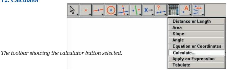
The calculator enables calculations to be carried out on values coming from the figure (measurements, displayed numbers, calculation results) or entered from the keyboard.
